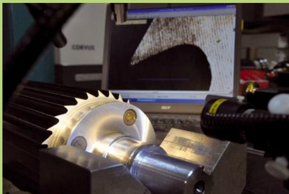
BKS carries out precision grinding to re-sharpen cutting rotors
